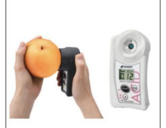
**Portable Meters** For acidity measurement, non destructive brix in fruit etc.
