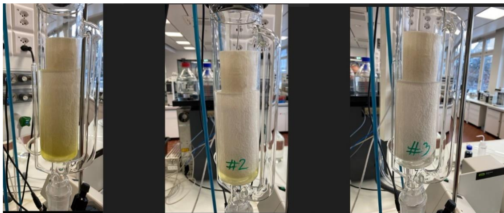
Picture 2: Extraction progression on a laboratory Rotavapor®. 1, 2 and 3 cycle
