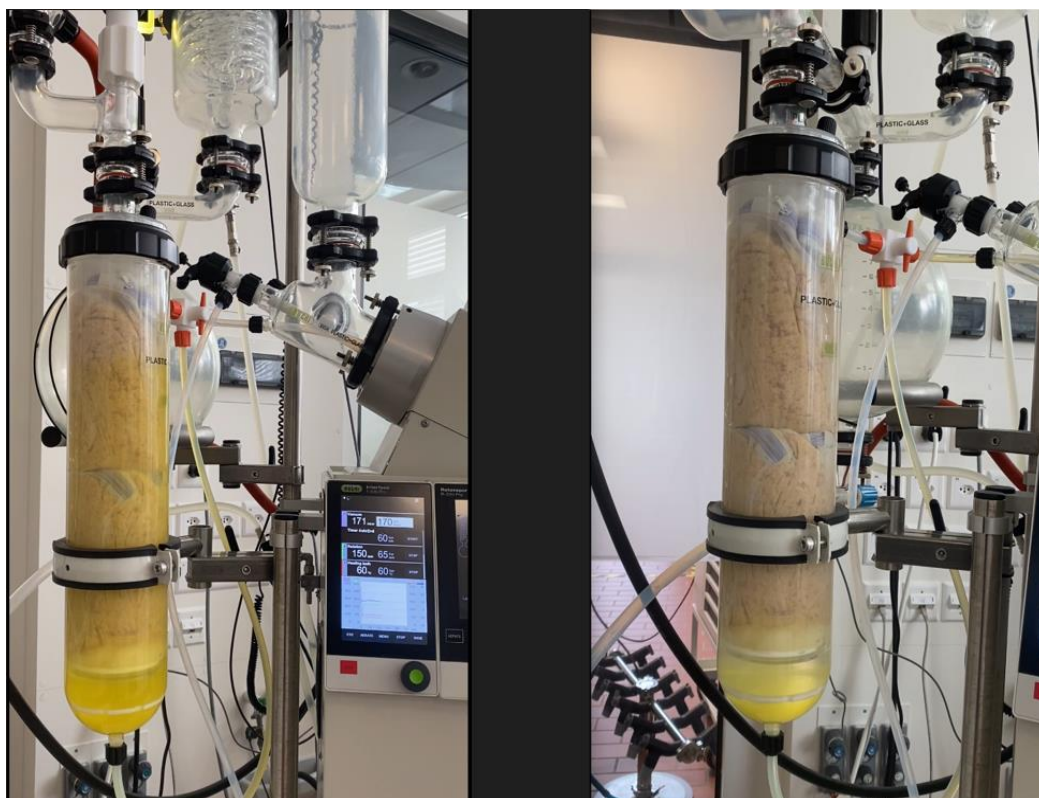
Picture 3: Extraction progression on an industrial Rotavapor® at time 0 and after 6 min
